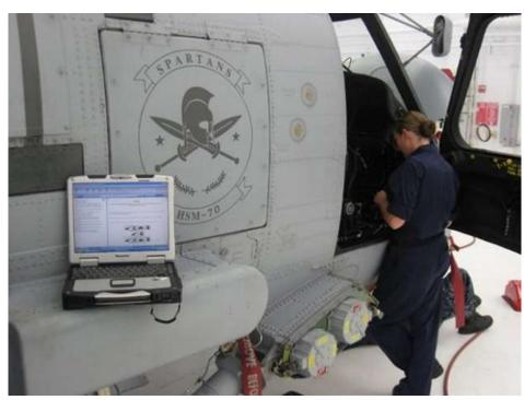
A PEMA in use during MH-60R maintenance at HSM-70. Photo courtesy of NAVAIR.
